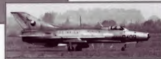
▲ Czech 'Fishbeds' Czechoslovakia was one of the first countries to acquire a licence to build MiG-21s. Known as CS-106s, these lacked the transparent panels behind the cockpit canopy.
